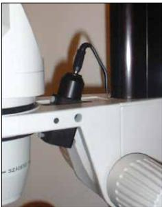
By using a special light source, Avalight, one can visualize the surface finish of a facet with very high contrast. Polishing lines can be observed more easily with this light source than with a classical light source.
